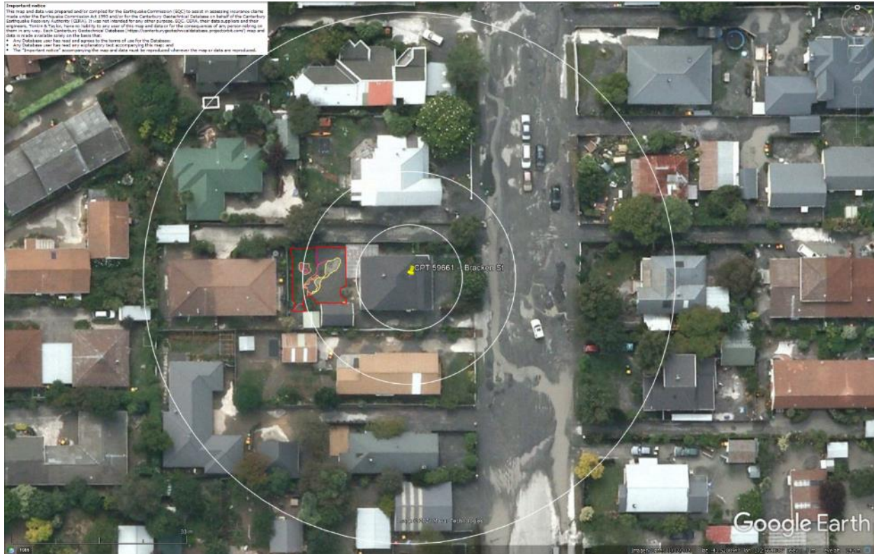
Figure 38: Aerial photograph showing the ejecta outline at the site for Feb-11 EQ.
